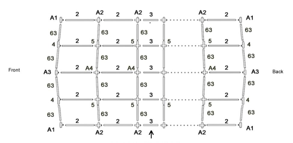
Extention tube of 1m (nr.3) should be placed in the third section.
