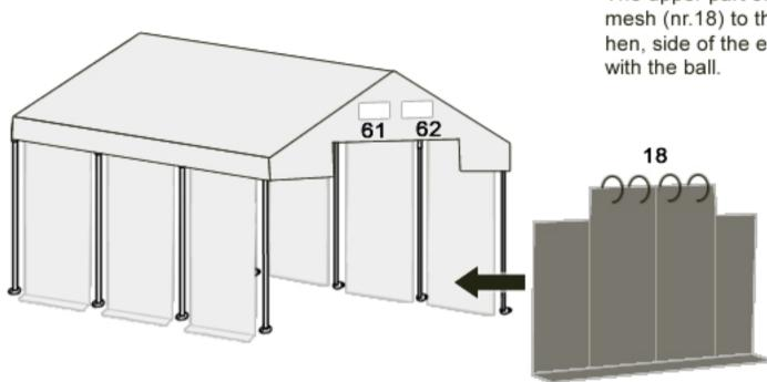
The upper part of the entrence install by the metal mesh (nr.18) to the horizontal pipes (nr.61 i nr.62). hen, side of the entrence attach with rubber bands with the ball.
