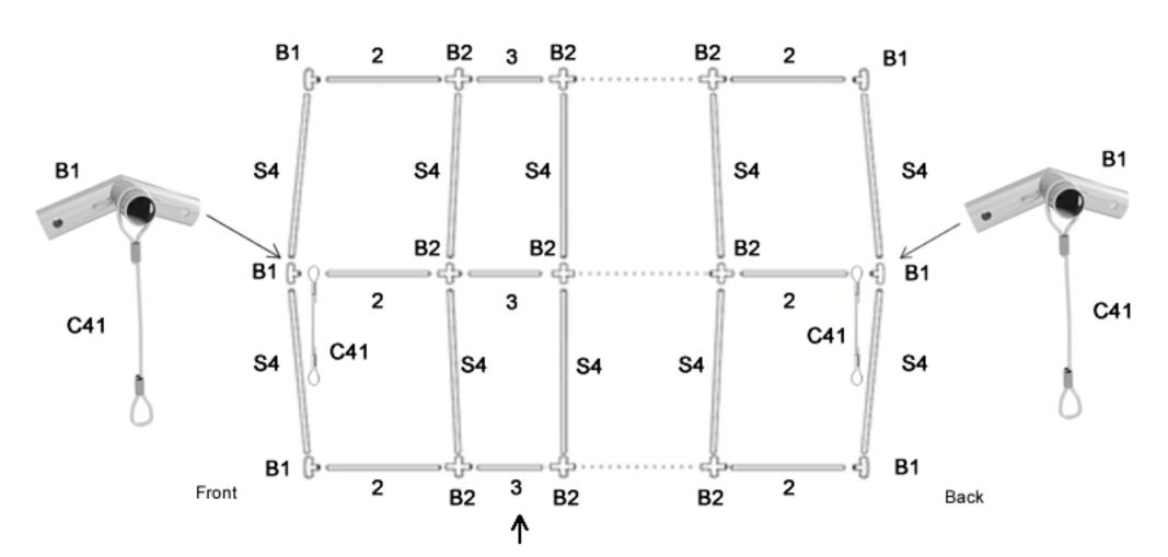
Pipe extending the tent by 1 meter (No.3) need to be placed in the second section.
