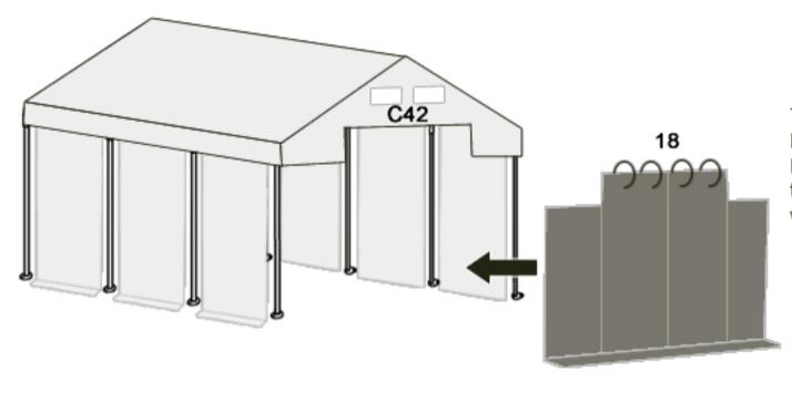
The upper part of the entrence install by the metal mesh(nr.18) to the horizontal links (nr.C42). Then, side of the entrnce attach with ruuber bands with the ball.
